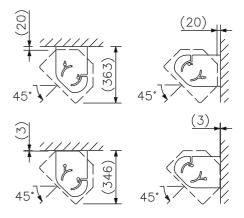
Dimension when the ES-0851 speaker is mounted so that the bracket faces outward.
